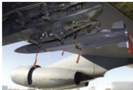
The Raytheon Miniature Air Launched Decoy Jammer (MALD-J) is designed to jam and confuse enemy air defenses.
